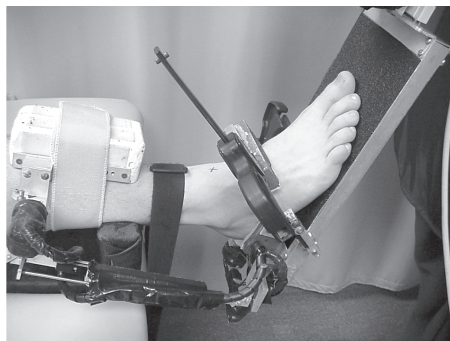
Figure. Setup for instrumented assessment of ankle joint laxity
